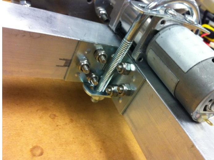
Figure 31: U shape nuts holding the gearbox to the bars.
